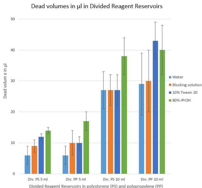
**Figure 2:** Average and error bars of dead volumes (in µl) in INTEGRA's polystyrene (PS) and polypropylene (PP) divided reservoirs (Div.). Tested solutions: Water, foaming Blocking solution, 10 % Tween 20 and 80 % isopropanol (iPrOH).
