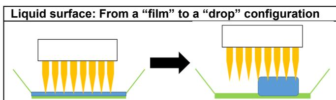
**Scheme 1:** Illustration of the tendency of a liquid to regroup and form a large drop instead of nicely spreading out in the deep trough all over its length when the liquid level lowers.
