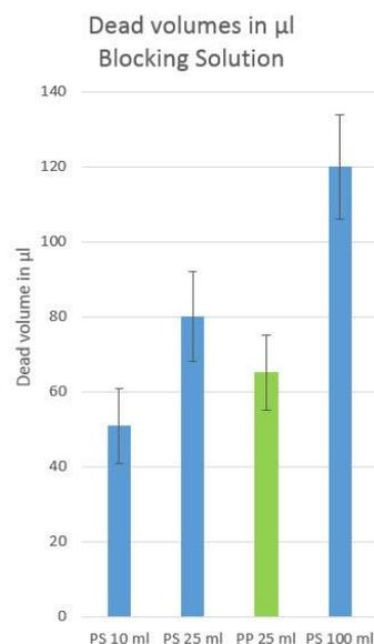
**Figure 1:** Average and error bars of dead volumes (in µl) in INTEGRA's polystyrene (PS) and polypropylene (PP) reservoirs starting from an initial volume of 36% of the nominal volume of the reservoirs.
